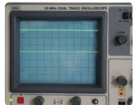
Figure 3 A display of two 1.5 V (3 V) cells in series connected to an oscilloscope
