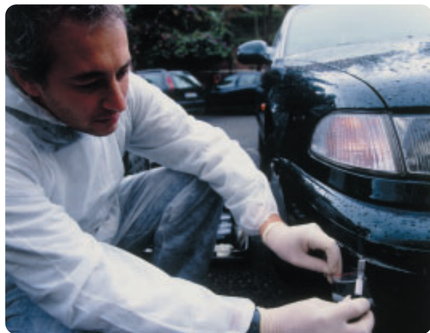
Figure 3 A forensic officer is using a scraping tool to remove paint that was transferred to the car from another vehicle when they collided.
