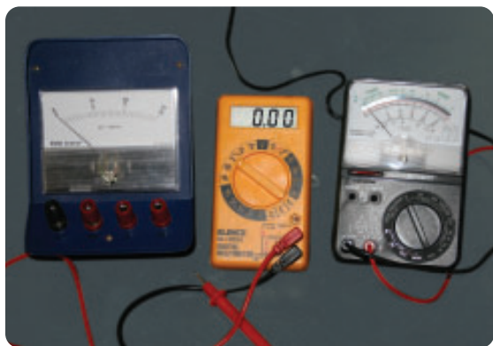
Figure 6 (From left to right) An analog voltmeter, digital multimeter, and analog multimeter
