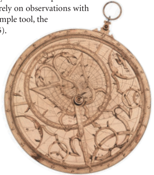
Figure 5 An astrolabe measures angles much like a protractor.
