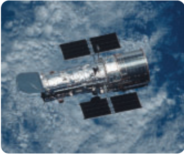
Figure 1 The Hubble Space Telescope over a cloudy Earth, with its protective flap open
