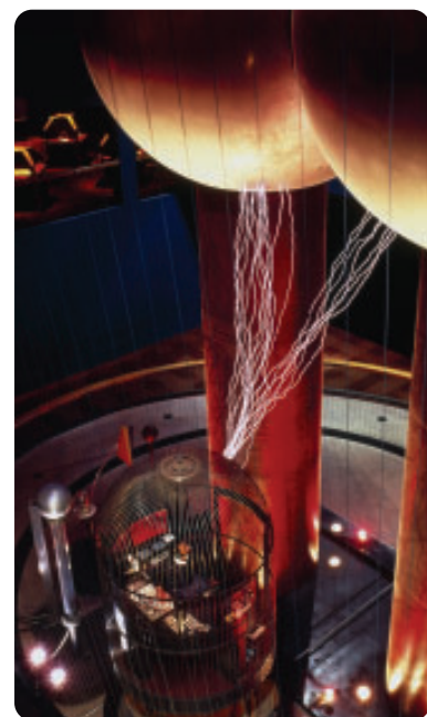
Figure 3 Michael Faraday showed that the charge stayed on the outside of a charged conductor, and did not affect anything enclosed within the conductor. Inside a Faraday cage, a person is safe from the static charge.
