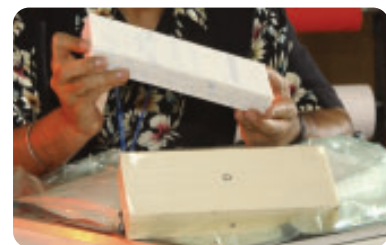
Figure 6 Blocks of reinforced polyethylene, like the one shown here, may be an important building material for future spacecraft.
