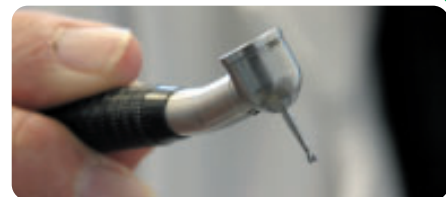
Figure 2 Many drill bits used by dentists have a diamond coating.
