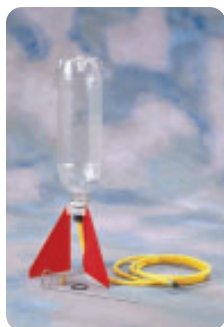
Figure 1 After adding water to the rocket, you can use the pump to increase the air pressure inside the rocket. What factors will control how high the rocket will go? Which of these factors could become independent variables?
