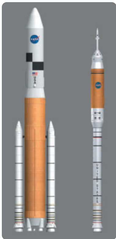
Figure 3 On the left is the Ares V at 110 m tall; Ares I is on the right. The I and V designations are a tribute to the Apollo program's Saturn I and V rockets, which were the first space vehicles built specifically for the piloted flights to the Moon.
