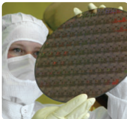
Figure 2 A wafer of silicon, from which dozens of microprocessors will be made
