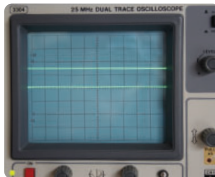
Figure 2 A display of a 1.5 V cell connected to an oscilloscope
