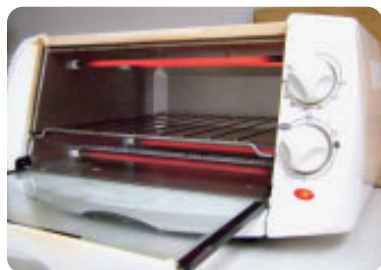
Figure 2 Nichrome is an alloy that has a melting point of 2550 °C. This melting point makes it useful for heating elements in toasters and ovens.
