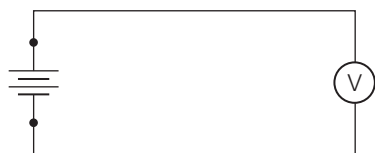
Figure 3 Measuring the voltage of a battery
