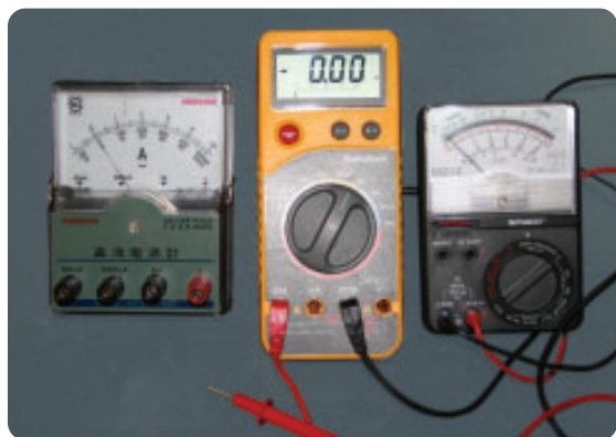
Figure 6 (From left to right) An analog ammeter, digital multimeter, and analog multimeter
